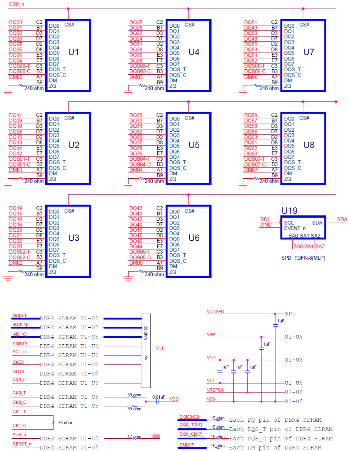
Figure 1 – Function Block Diagram_SCC08GU03C2F1C-32AA
